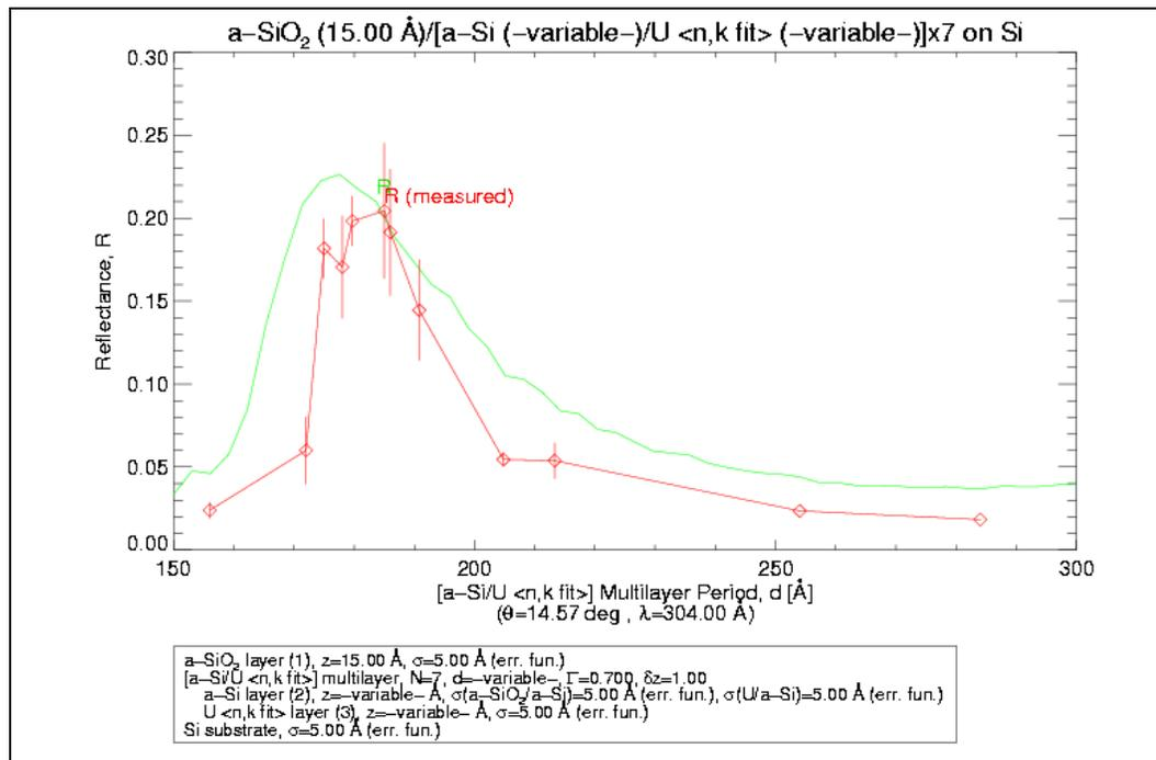
Figure 26: Measured and Calculated Reflectivities with amorphous silicon cap at 304 Å
