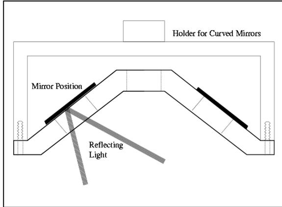
Figure 12: Side View of Mirror Holder
