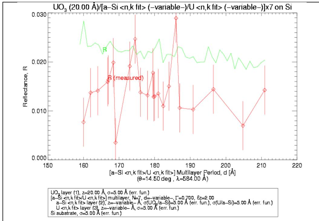
Figure 28: Measured and Calculated Reflectivities with uranium oxide cap at 584 Å
