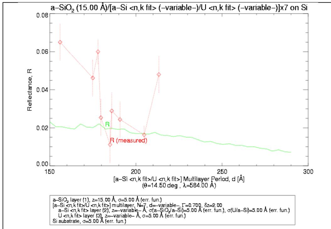
Figure 29: Measured and Calculated Reflectivities with amorphous silicon cap at 584 Å
