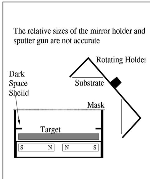
Figure 2: Side View of Sputter Setup
