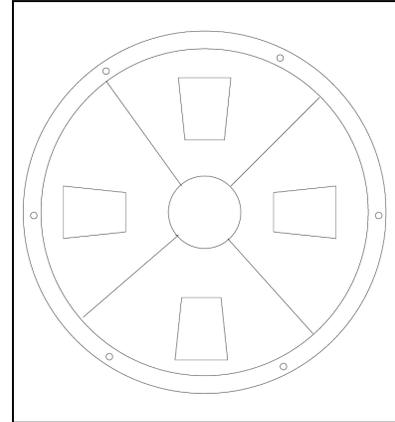
Figure 13: Top View of Mirror Holder
