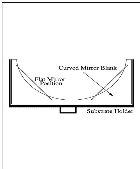
Figure 4: Relative Positions of Flat and Curved Substrates
