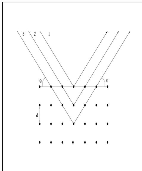
Figure 5: Bragg Diffraction
