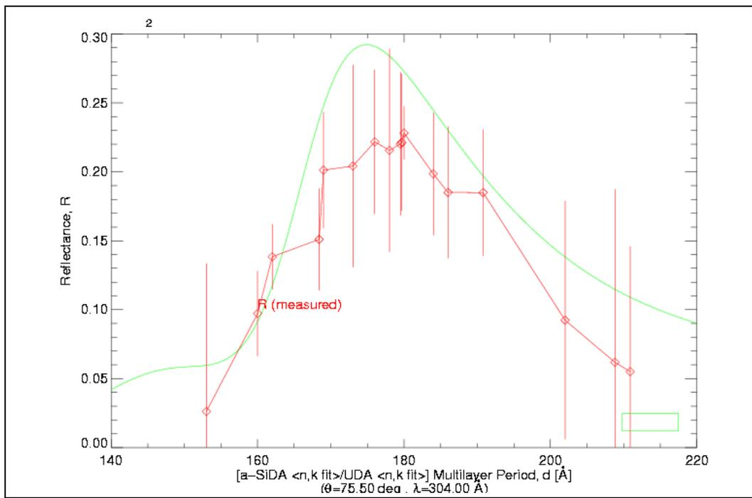
Figure 27: Measured and Calculated Reflectivities with uranium oxide cap at 304 Å
